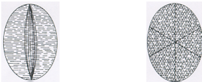
Figure 1.2 (Left). Chatoyancy. Orientation of inclusions at right angles to the beam of light. (Right) Star effect produced by intersection of three sets of inclusions 120^\circ apart.
